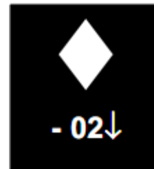
Symbol of a non-threat proximity traffic (full white or blue diamond) Separation < 1200 ft or distance < 6 NM
