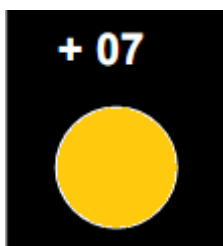
Symbol of a Traffic Advisory - TA alert (full orange or amber circle)
