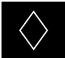
Symbol of non-threat traffic of unknown altitude (empty diamond with white or blue borders) Separation > 1200 ft or distance > 6 NM
