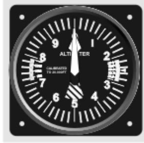
In aircraft, an aneroid barometer measures the atmospheric pressure from a static port outside the aircraft. Air pressure decreases with an increase of altitude—approximately 100 hectopascals per 800 meters or one inch of mercury per 1000 feet near sea level.
