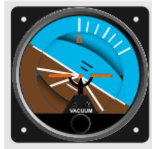
There is also a miniature aircraft (orange line) and horizon bar representation. The horizon is displayed using a white line which separates the instrument in two parts:
