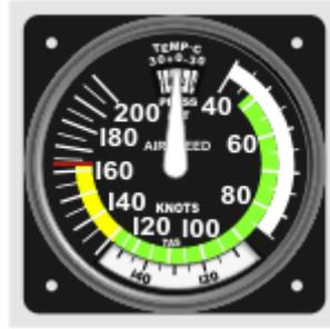
The direct instrument reading obtained from the airspeed indicator, uncorrected for variations in atmospheric density, installation error, or instrument error. Manufacturers use this airspeed as the basis for determining airplane performance.
