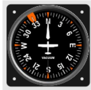
The heading indicator is fundamentally a mechanical instrument designed to facilitate the use of the magnetic compass. Errors in the magnetic compass are numerous, making straight flight and precision turns to headings difficult to accomplish, particularly in turbulent air.
